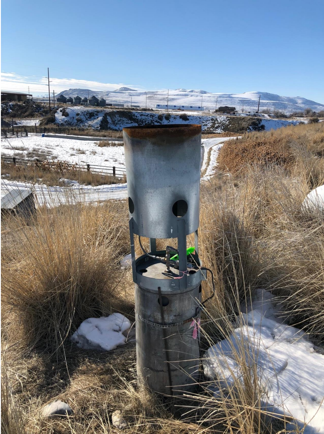
Figure 1.2: Cloud seeding generator that is located at Bear River City, UT turn on during the suitable seeding condition targeting the orographic clouds over the mountain.
