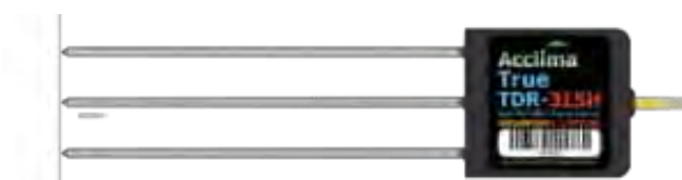
Figure 3: The Acclima TDR 315 sensor used to collect soil moisture data.
