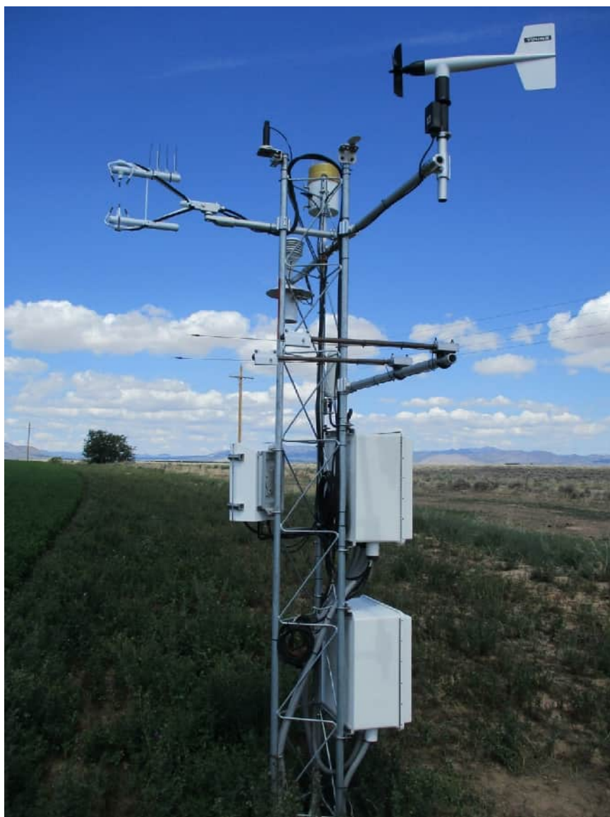
Figure 1. Eddy covariance tower sited at north edge of the alfalfa.
