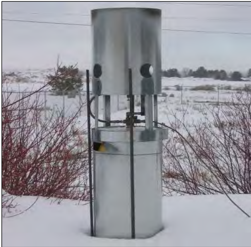
Figure 2.2 Manually operated cloud seeding generator
