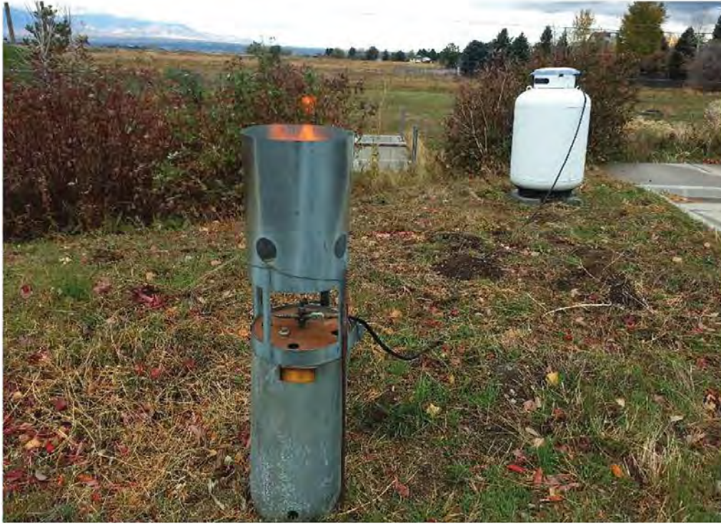
Fig. 4. Ground based, manually operated Silver Iodide nuclei generator.
