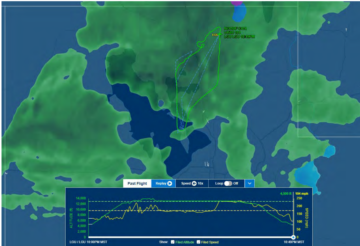
Figure 5.4. Flight track from seeding mission on November 6, 2023. Lower graph indicates altitude of plane (green) and speed of plane (yellow) during flight. Green and blue shading in background is radar image at time of image capture. Courtesy of FlightAware.com website.
