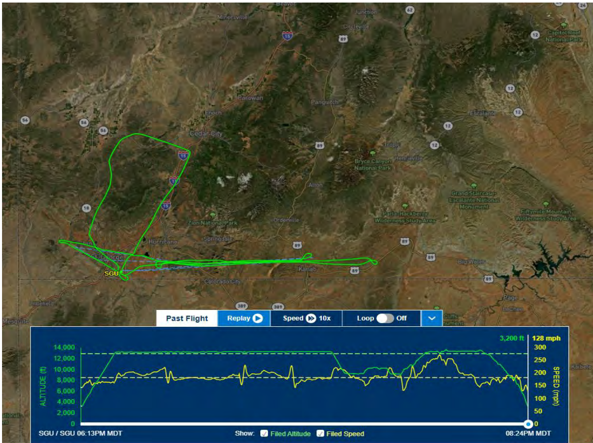
Figure 3.2. Cumulative flight track from FlightAware.com from a seeding flight over far southern Utah on March 30, 2024. Bottom quarter of image shows altitude (green line) and speed (yellow line) during the flight.
