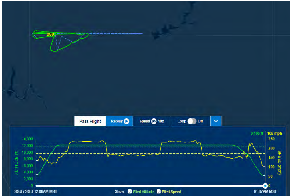
Figure 5.8. Flight track from seeding flight on January 7, 2024. Lower graph indicates altitude of plane (green) and speed of plane (yellow) during flight.
