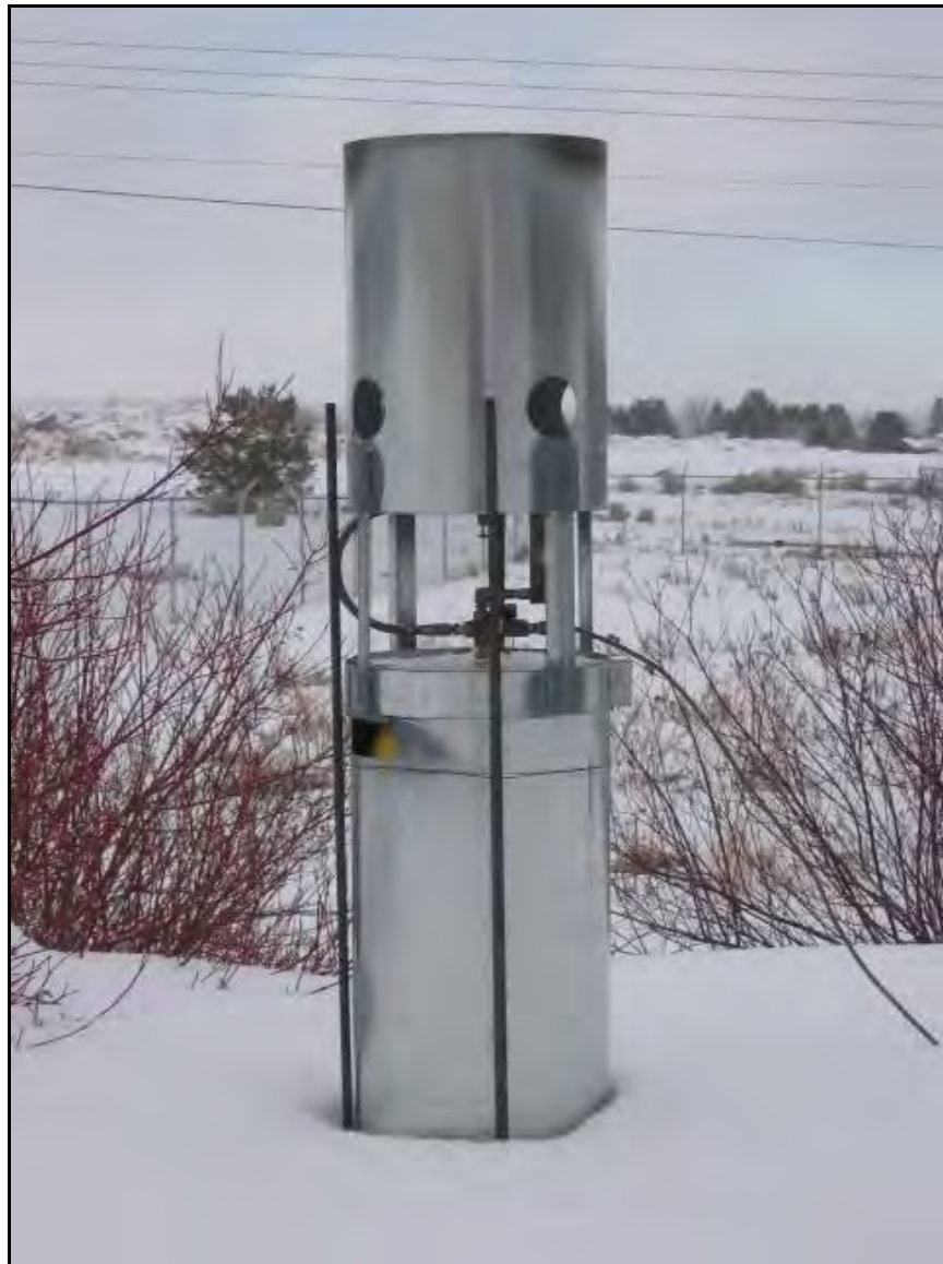
Figure 2.2 NAWC manually operated cloud nuclei generator (CNG)
