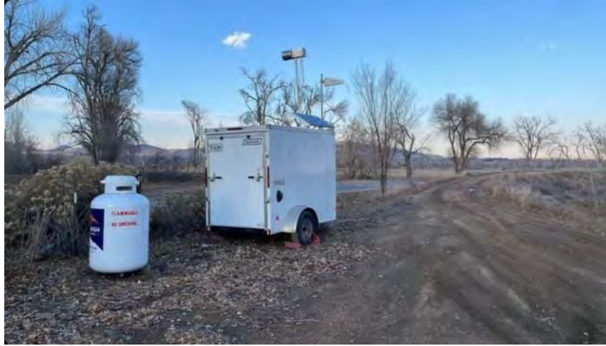
Figure 2.3 Photo of a NAWC remotely operated Cloud Nuclei Generator (CNG)
