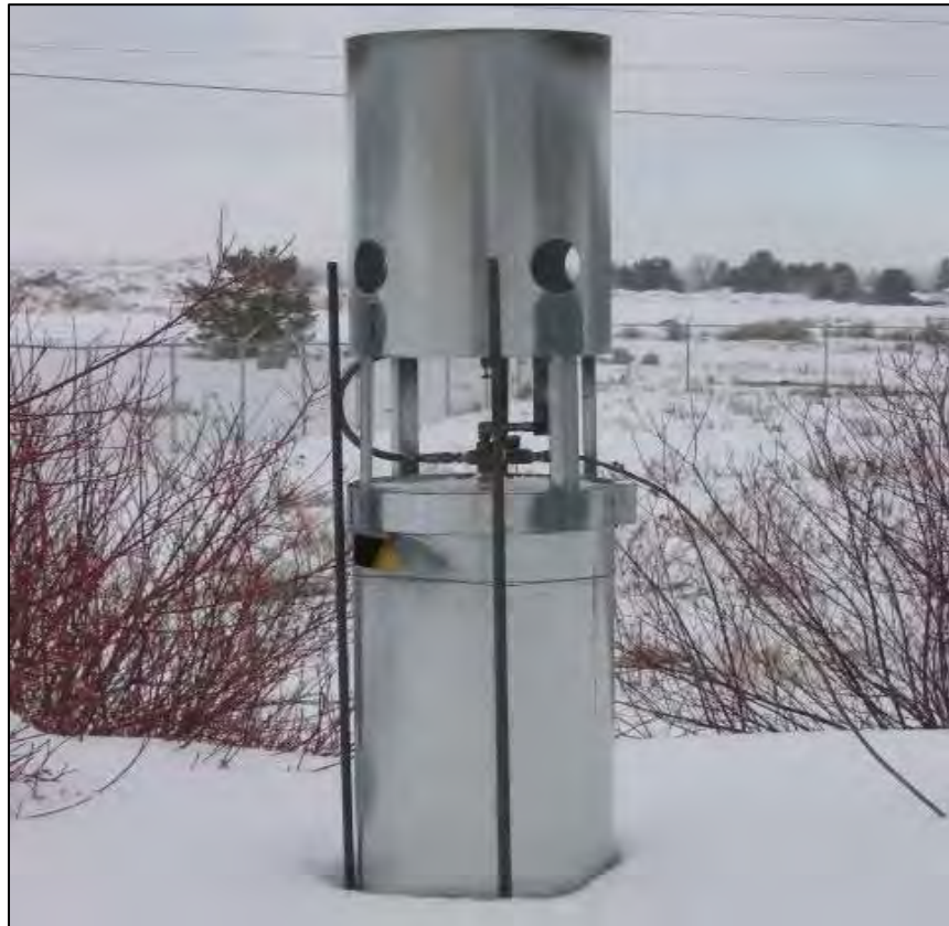
Figure 2.2 Manually operated cloud seeding equipment
