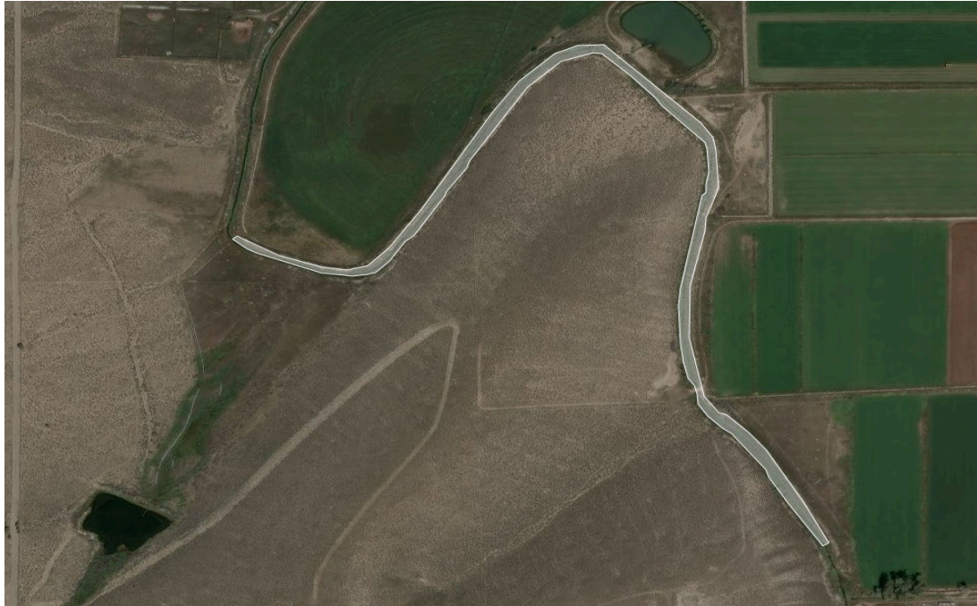
Figure 26: Digitized canal corridor used for off-farm depletion analysis and OpenET data extraction
