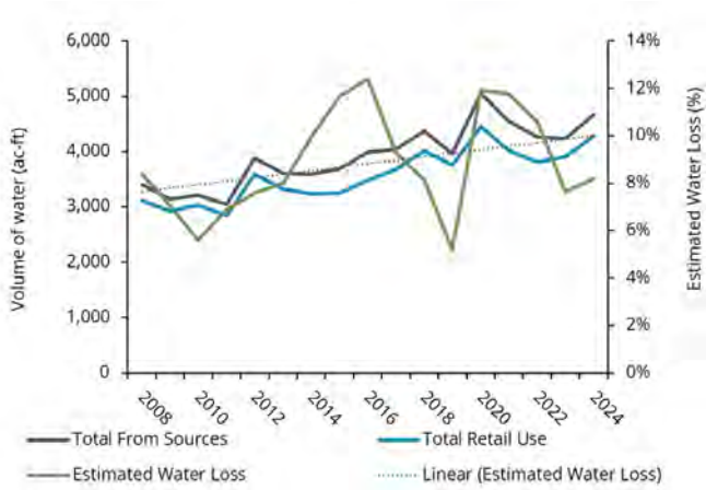
Figure 12- WaterPro Secondary Source, Use, & Estimated Water Loss
