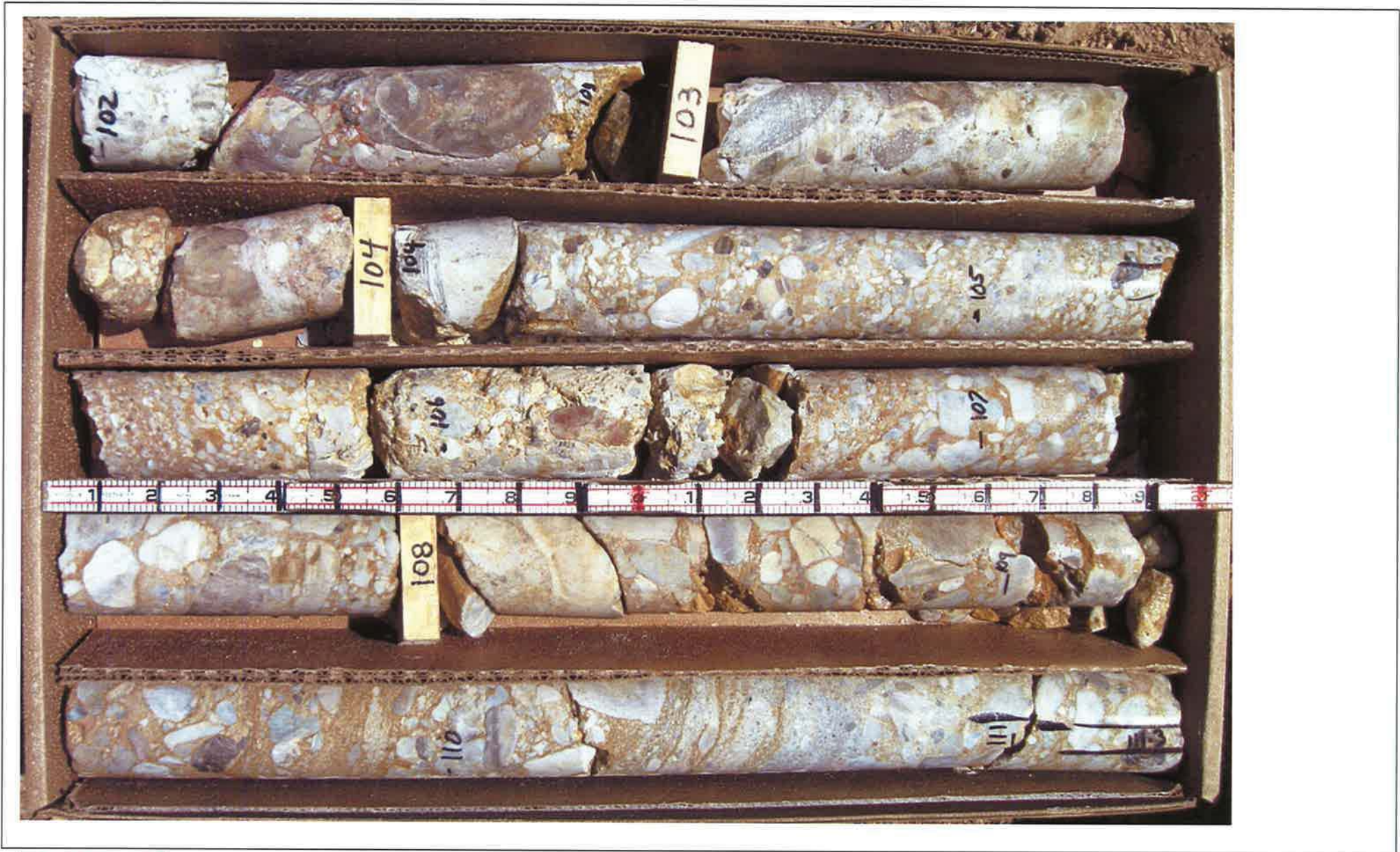
Figure Drill Hole #09-FB-9 Core Photos Wet Drilled at a dip of 60 degrees from Horizontal (30 degrees from Vertical) Project HCH Forebay South Dam Site, WCWCD Location Washington County, Utah
